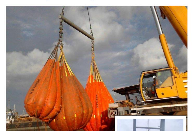
Capacities of 1t - 35t allow WaterLoads to be used singly or in clusters to produce test loads of upto 100t on one hook. Multiple clusters can be used for higher loads.
